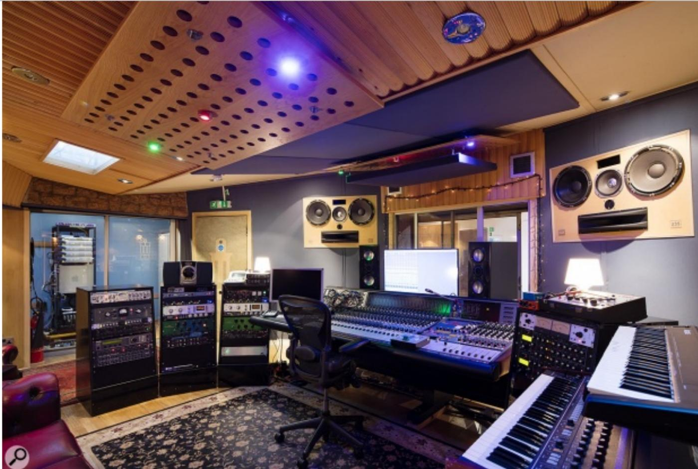
The control room is based around a 32-input Neve 8232 console.
